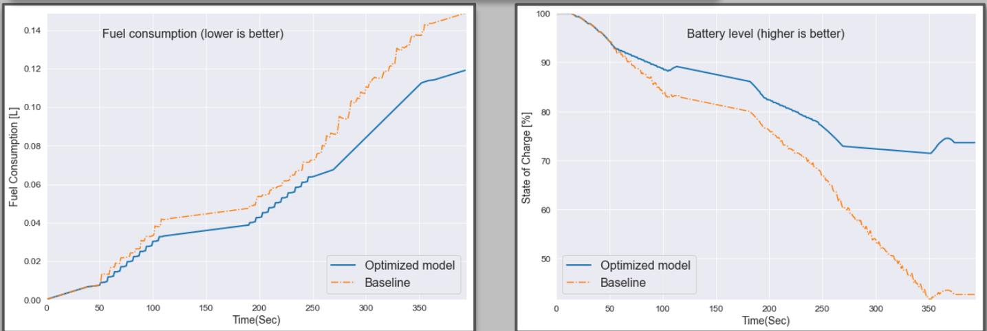
The fuel consumption (left panel) and the battery state of charge (right panel). The optimized, trained, model (blue solid line) is presented alongside the baseline (orange dash-dotted line). Visible is that after the training is completed, the optimized controller gives better performance both in terms of fuel consumption and state of charge. Particularly the fuel usage drops by 20% while the battery charge is increased by 72%.
