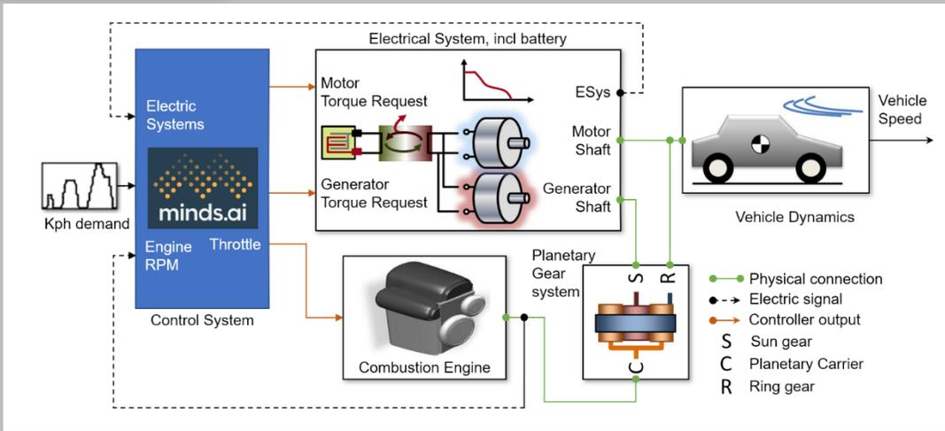
Hybrid electric vehicle drive line schematic, based on the design of [1]
