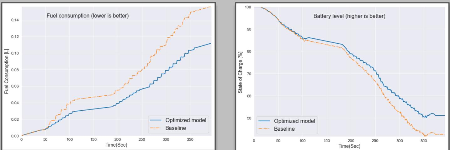
As Figure 2, but now with a different fuel vs battery preference ratio. In this example the fuel usage drops by 29% while the battery charge improves by 20%. This shows it is possible to use DeepSim to tune the controller to meet different objectives.
